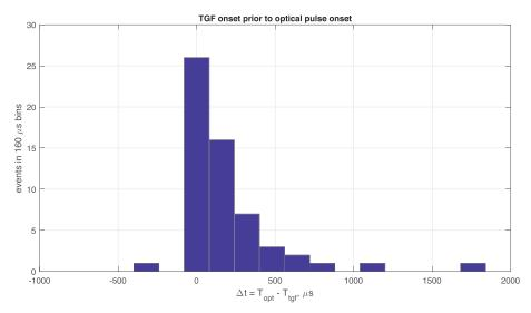
**Figure 7.** Distribution of  $\Delta t$  between the onset of the TGF and the onset of the optical pulse for 58 TGF events where the optical pulse could be identified. Bin size is 160 μs consistent with the ±80 μs relative timing uncertainty between the two observations. Positive  $\Delta t$  means that the onset of the TGF is before the onset of the optical pulse.
