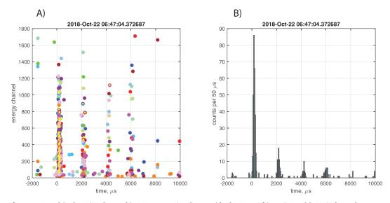
Figure 8. A multipulse TGF observed in HED on 22 October outside the West African Coast. (a) ADC channel versus time. (b) counts in  $50 \mu s$  bins versus time.
