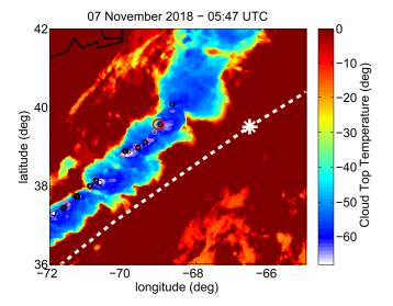
**Figure 9.** The storm system for Terrestrial Gamma-ray Flashes (TGF) number 4. The circles and the pluses are -CG and +CG respectively, detected within 5 min around the TGF (the pink before and the black ones after). The red circle is the associated stroke. The dashed line shows the International Space Station trajectory and the white star marks its position at the time of the detection.
