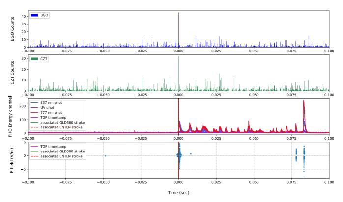
**Figure 7.** The Bismuth-Germanium Oxide (High Energy Detector (HED)), CZT (Low Energy Detector (LED)), optical and radio data for the event of 2018-Nov-07. The bin size for HED and LED histograms is 100  $\mu$ s.
