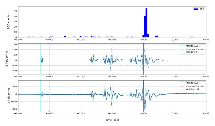
**Figure 10.** Top: the Bismuth-Germanium Oxide lightcurve, with a bin size of 50  $\mu$ s. Middle: the radio waveform recorded by Earth Networks Total Lightning Network for the associated stroke. Bottom: the radio waveform as recorded by the authors (Füllekrug). Here the Terrestrial Gamma-ray Flashes is matched to the second sferic based on the largest peak current (see main text).
