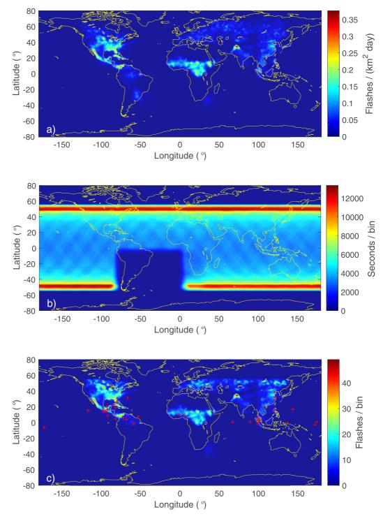
**Figure 2.** (a) Global lightning flash density, from Lightning Imaging Sensor/OTD global climatology maps. (b) Atmosphere Space Interaction Monitor's exposure, with the South Atlantic Anomaly very visible. (c)  $F_{ij}^{(m)}$ , as defined in the main text, with the Terrestrial Gamma-ray Flashes detected in the corresponding period (red crosses). Here we show the month of July, 2019 as an example. Bin size in all maps is  $0.5^{\circ} \times 0.5^{\circ}$ .
