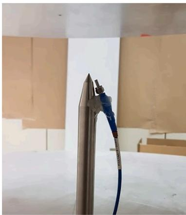
Fig. 2. Picture of the optical fiber pointing to the tip of the rod.
