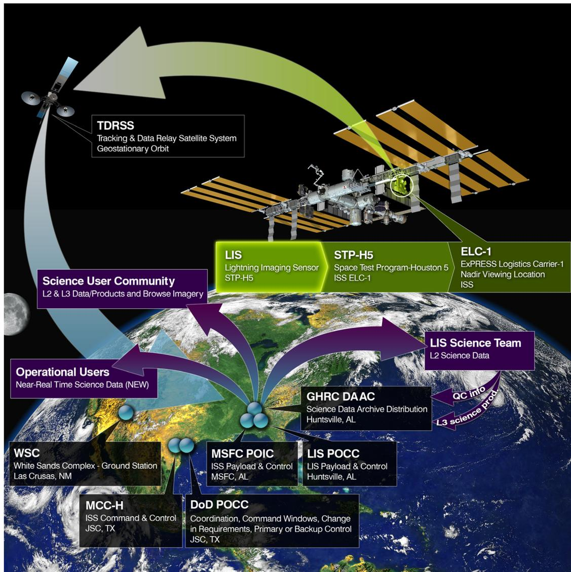
**Figure 1.** Visualization of the ISS LIS instrument, its location on the ISS, as well as its data collection, processing, and distribution.
