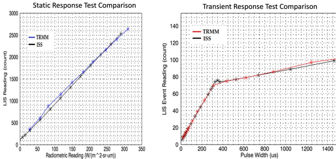
**Figure A1.** The close comparison between the original TRMM LIS calibration (OC; labeled TRMM) and the retest calibration (RC) of ISS LIS (labeled ISS). For a representative subset of the instrument’s FOV. (left) Static response test. (right) Transient response test.
